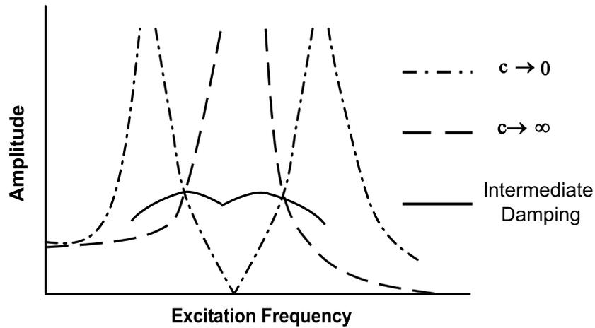
**Figure 3:** Theoretical response for different amounts of damping
