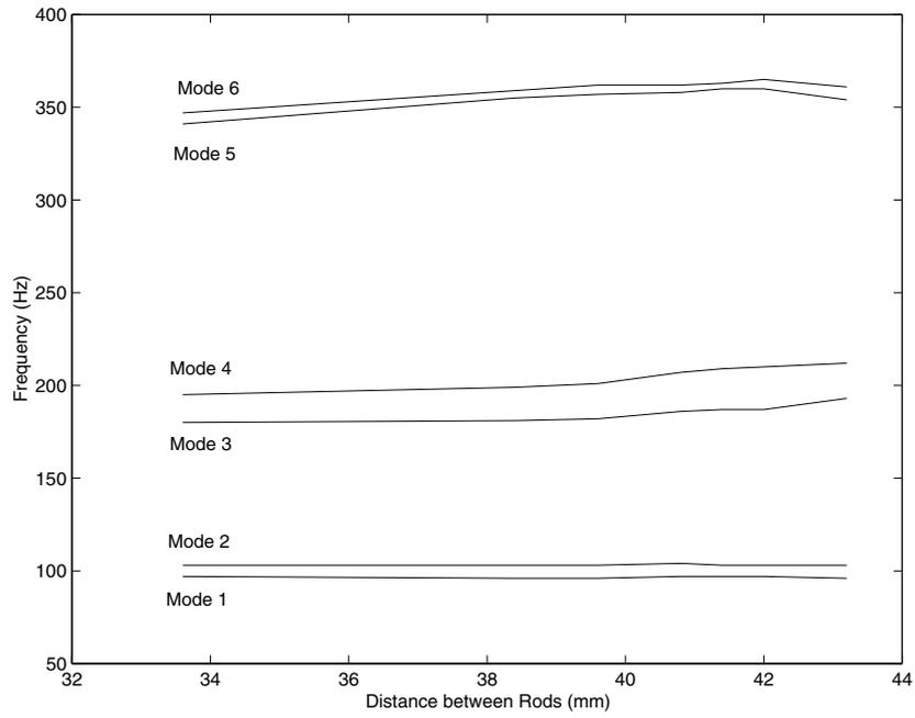
**Figure 6:** Tuning Mode three and four
