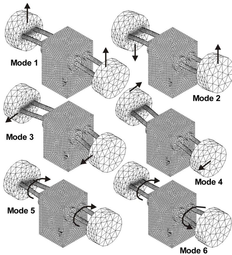
**Figure 5:** Absorber Modes. Clockwise from top left, mode 1,2,3,4,5 and 6. Modal frequencies 95, 105, 196, 204, 295 and 304 Hz respectively.
