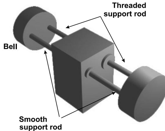
**Figure 4:** The dual mass absorber
