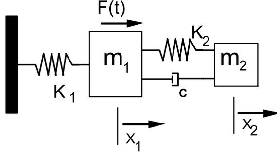
Figure 1: Primary system and absorber schematic
