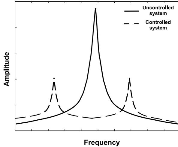
**Figure 2:** Frequency response with a well tuned absorber
