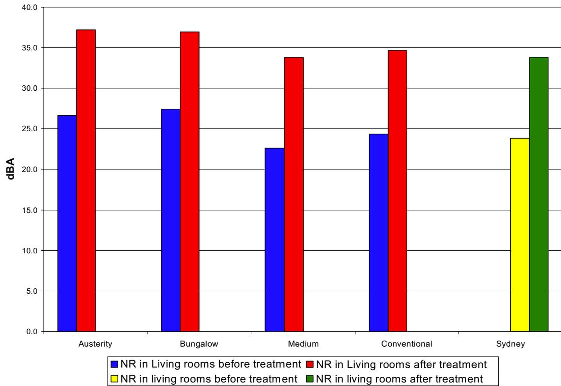
**Figure 1:** Comparison between the average improvement in noise reduction in the living rooms of the treated residences gained during AANIP and SANIP
