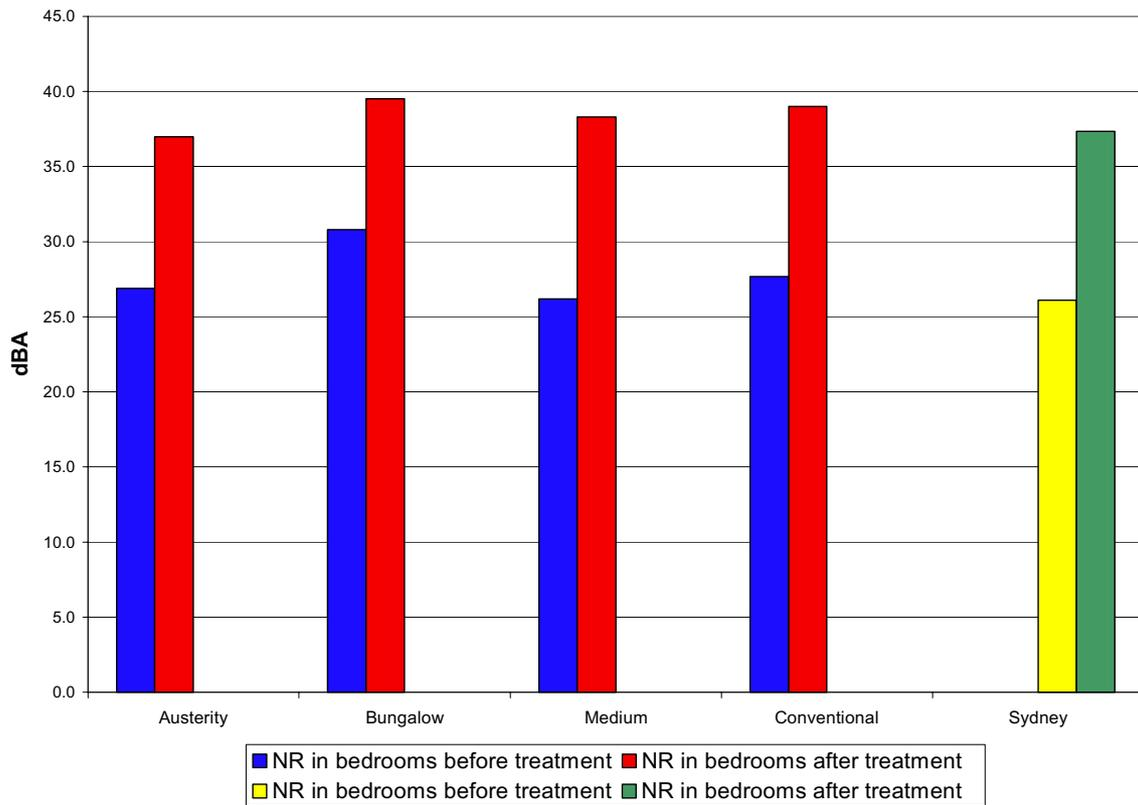
**Figure 2:** Comparison between the average improvement in noise reduction in the bedrooms of the treated residences gained during AANIP and SANIP
