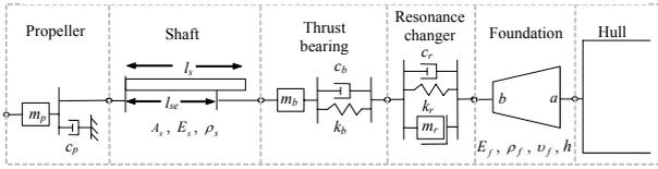
**Figure 2.** Modular representation of propeller-shafting model connected to the submarine hull.
