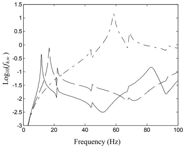
**Figure 7.** Force transmissibility (--- no RC, ..... with 1 optimal RC, — with 2 optimal RCs).
