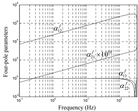
**Figure 3.** Four pole parameters of the foundation  $\mathbf{a}^f$ .
