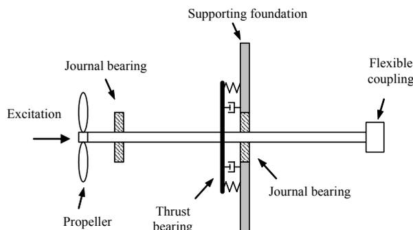
Figure 1. Simple schematic of the propeller-shafting system (Pan *et al.* 2002).
