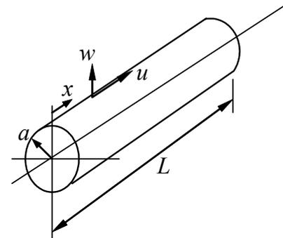
Figure 4. Coordinate system of a cylindrical shell.
