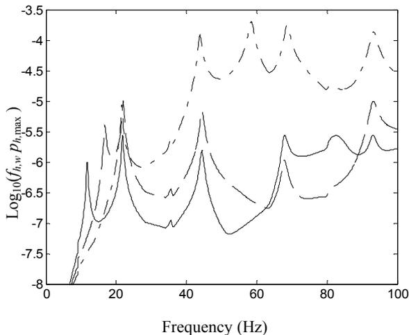
**Figure 8.** Radiated sound pressure (--- no RC, ..... with 1 optimal RC, — with 2 optimal RCs).
