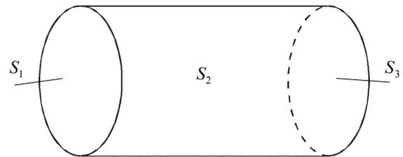
Figure 5. Surface areas of the end plates and cylindrical shell.
