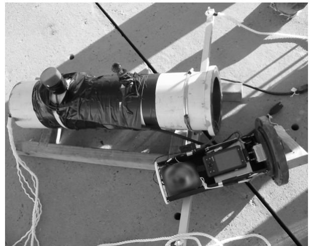
Figure 3. Deep sea housing (left) and associated recorder and modem receiver components (right).
