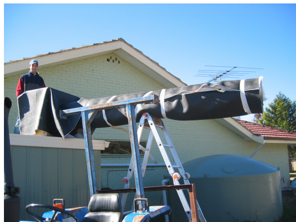
Source: Daniel Potente Figure 4. 305 mm duct - loaded vinyl wrapped
