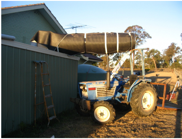
Source: Daniel Potente Figure 5. 600 mm duct - loaded vinyl wrapped
