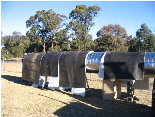
Source: Daniel Potente Figure 6. 915 mm duct - loaded vinyl wrapped
