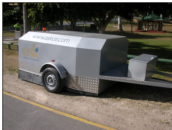
Figure 1: ROAD-EAR CPX Trailer Developed by ASK Consulting Engineers
