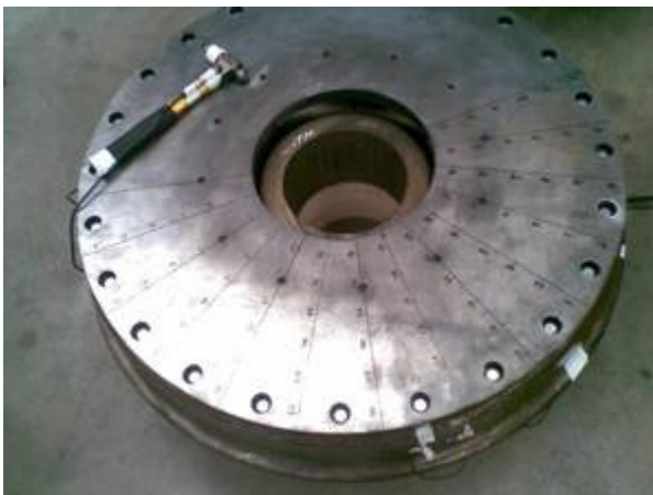
Figure 13 Impact modal test layout, showing measurement grid on the constrained layer and reference accelerometer location shown.
