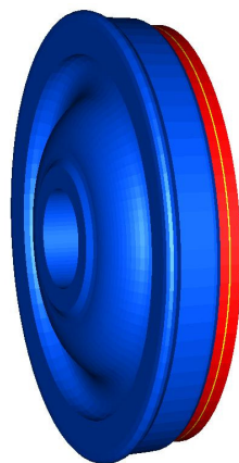
Figure 9 FEM of wheel with baseline CLD treatment
