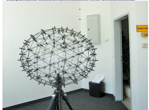
Figure 10: measurement in empty office room, testing common shredder (5dB dynamic)
