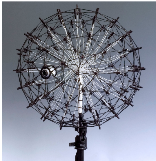
Fig. 5: Spherical acoustically transparent arrays with 48 channels and 120 channels and a built-in video camera
