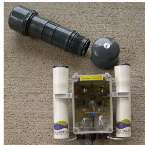
Figure 3. NGNRM dugong alarm casing with 2 sound generating inserts on a charger locally made in the fishery region.
