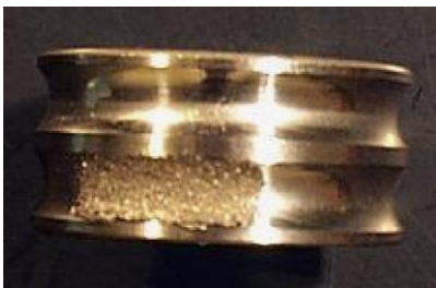
Figure 3: Extended inner race fault (Sawalhi and Randall, 2008b)
