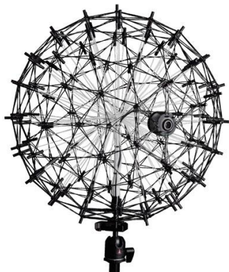
Figure 1 – 3D - microphone array with 120 spherically distributed microphones for the analysis of interiors
