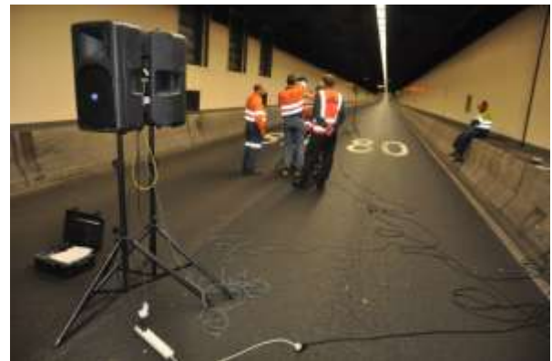
Figure 9. Experimental setup, Sydney harbour tunnel (width 8.35 m,height 4.98 m, length 2.8 km)
