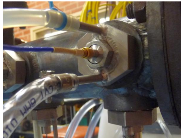
Figure 2: Photograph showing the custom made water-cooled jackets for PCB microphones.
