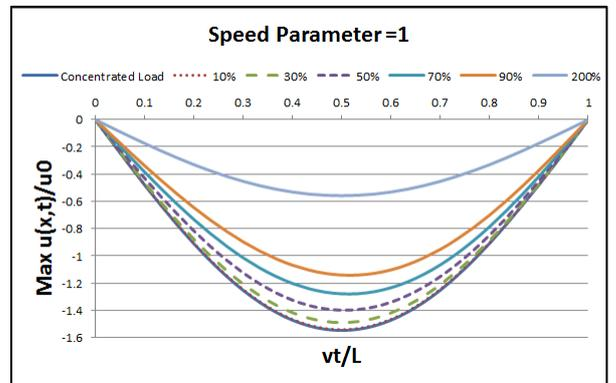
Figure 13: Normalised Deflection  $Max u(x,t)/u_0$  for Various Distributed Load Lengths at Speed Parameter of 1.0
