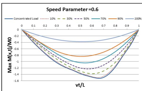
**Figure 16: Normalised Bending Moment  $\text{Max } M(x,t)/M_0$  for Various Distributed Load Lengths at Speed Parameter of 0.6**
