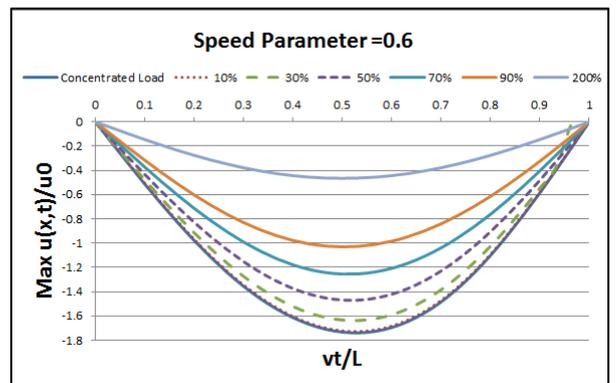
Figure 14: Normalised Deflection  $Max u(x,t)/u_0$  for Various Distributed Load Lengths at Speed Parameter of 0.6
