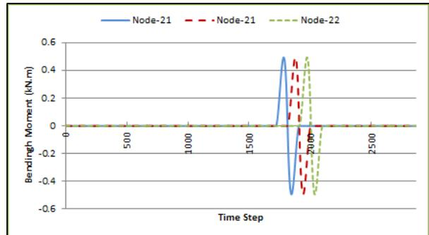
**Figure 9: Bending Moment-Time Step Graph for Nodes-20/21/22 for the Concentrated Load**
