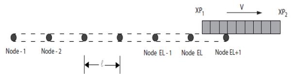
**Figure 19: Departure of Moving Load from the Simply Supported Beam (Distributed Load Covers Part of the Last Element)**
