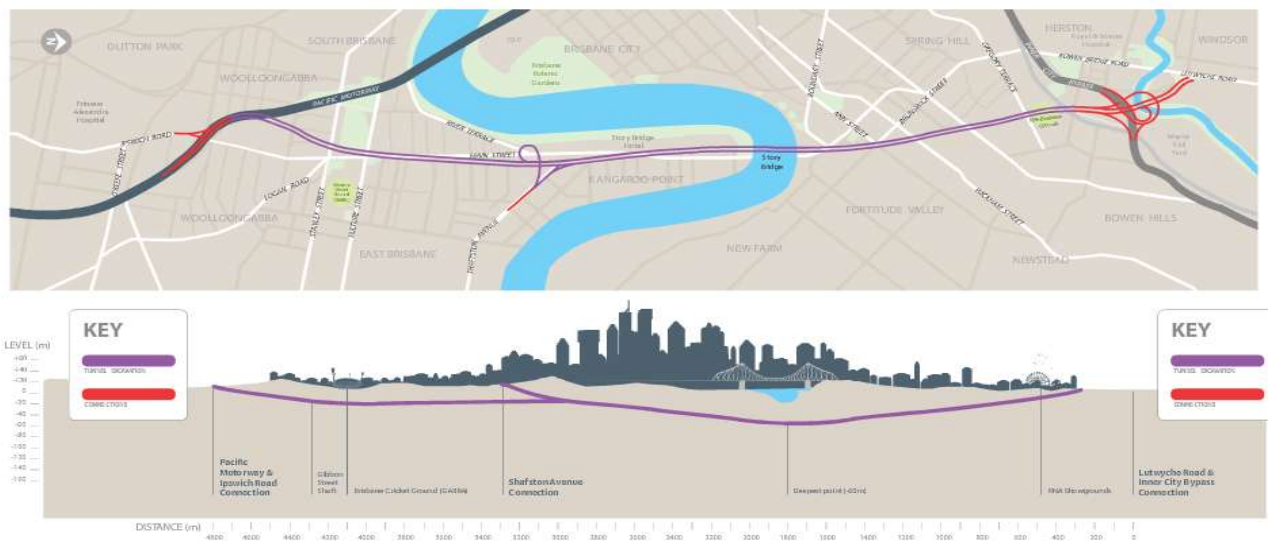
Figure 1: Location and alignment of the Clem7 Tunnel
