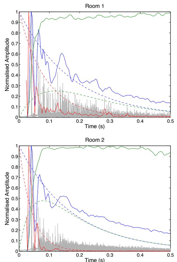
Figure 2 Analysis of simulated RIR from MCRoomSim of rooms 1 & 2 from Hanyu. ETC of RIR in grey, dashed green line shows  $P_d(t)$ , dashed red line shows  $P_{spec}(t)$ , dashed blue line shows  $P_a(t)$ , blue line shows  $\sigma$ , red line shows kurtosis, green line shows NED. Window size 24 ms, step size 4 ms.
