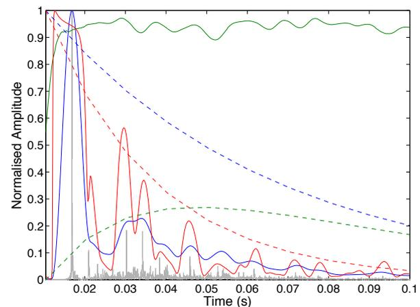
Figure 4 An example of the analysis of room A816 in reverberant state. ETC of RIR in grey, dashed green line shows  $P_d(t)$ , dashed red line shows  $P_{spec}(t)$ , dashed blue line shows  $P_a(t)$ , blue line shows  $\sigma$ , red line shows kurtosis, green line shows NED. Window size 10 ms, step size 0.2 ms.
