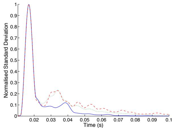
Figure 5 A comparison of the standard deviation analysis for room A816 in three states, reverberant (red dashed line), diffuse (green dotted line) and anechoic (solid blue line). Window size 10 ms, step size 0.2 ms.
