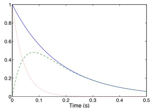
Figure 1 Typical energy decay curves after Hanyu. The dashed line shows the evolution over time (in seconds) of energy in the room attributed to diffuse reflections,  $P_d(t)$ . The dotted line shows energy attributed to specular reflections,  $P_{spec}(t)$ . The solid line shows the combined energy in the room from all reflections,  $P_a(t)$ .
