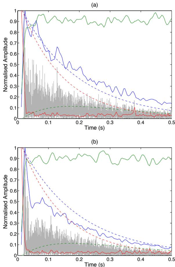
Figure 3 Analysis of reverberation room with no diffusers (a) and 15 diffusers (b). ETC of RIR in grey, dashed green line shows  $P_d(t)$ , dashed red line shows  $P_{spec}(t)$ , dashed blue line shows  $P_a(t)$ , blue line shows  $\sigma$ , red line shows kurtosis, green line shows NED. Window size 24 ms, step size 4 ms.
