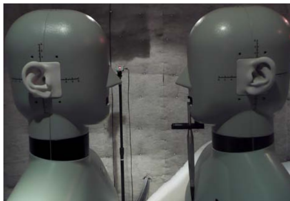
Figure 1. Photograph of the pair of anthropomorphic manikins that were employed to make measurements between the orally-radiated source (right manikin) and the ear canal entrance of the receiver (left manikin) as that receiver is rotated through a 180 deg. range of azimuth angles. Note the presence of a microphone at the mouth opening of the source manikin (on the right) that could be used to examine directly the oral-to-ear transfer function between manikins.
