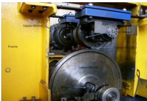
Figure 3. Front view of the two disk rolling contact test rig
