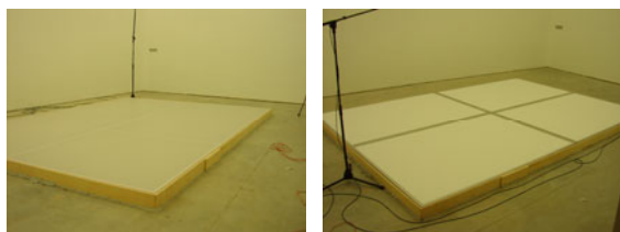
Figure 5. Experimental set-up of the stretched ceiling / foil. Left: one single sheet of 12 m 2 Right: four sheets of 3 m 2 each.
