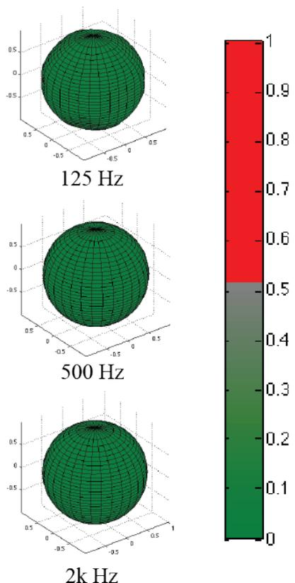
**Figure 4.** Directivity patterns for 0<sup>th</sup> order spherical harmonic simulation. Colour-coding shows absolute error from normalised values.
