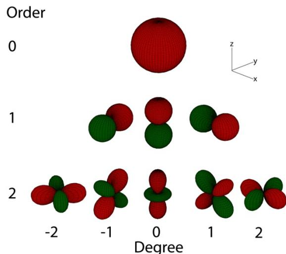
**Figure 3.** Visualisation of spherical harmonics, up to the second order. Colour indicates phase.
