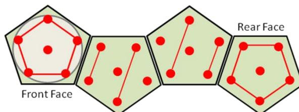
**Figure 2.** Microphone positions (red dots) expressed as equivalent angles from the dodecahedron centre on each of the four non-redundant faces of the dodecahedron (shown as a partial net). Redundant microphone positions are linked by red lines.
