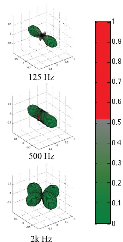
**Figure 6.** Directivity patterns for 2<sup>nd</sup> order spherical harmonic simulation. Colour-coding shows absolute error from normalised values.
