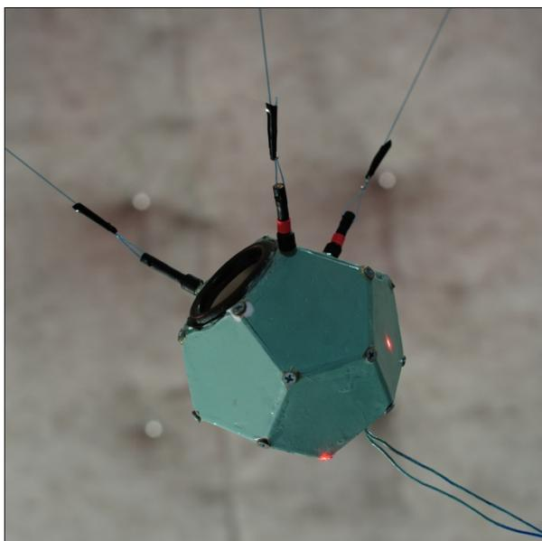
**Figure 1.** Photograph of the prototype sound source, showing the magnetic suspension system and the laser-guided positioning (the red spots).
