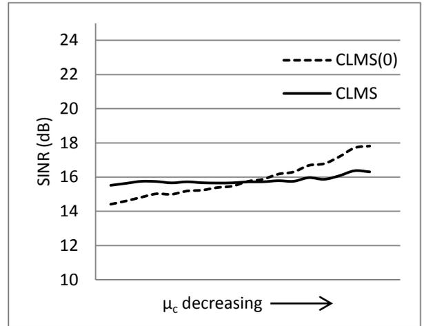
Figure 5. Scenario 4 - Look-direction mismatch, with model error
