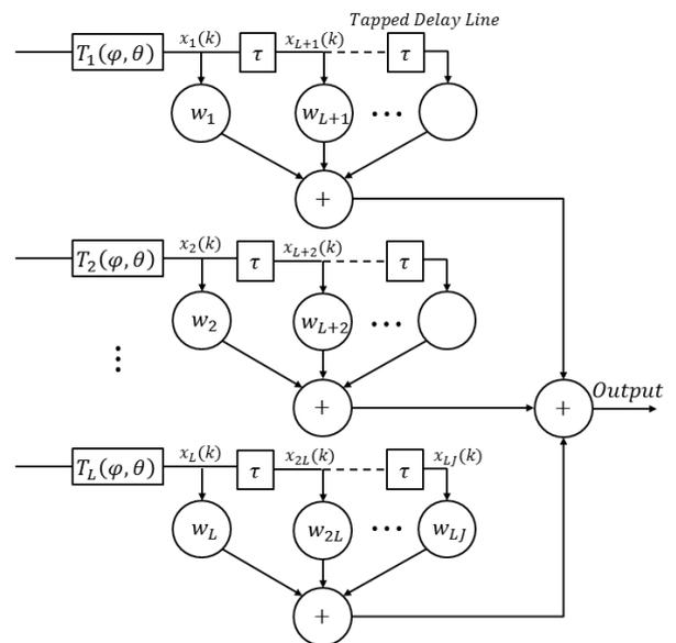
Figure 1. Broadband Beamformer Structure
