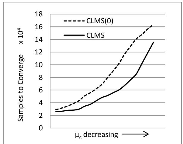
Figure 6. Number of samples required for adaptive weights to converge
