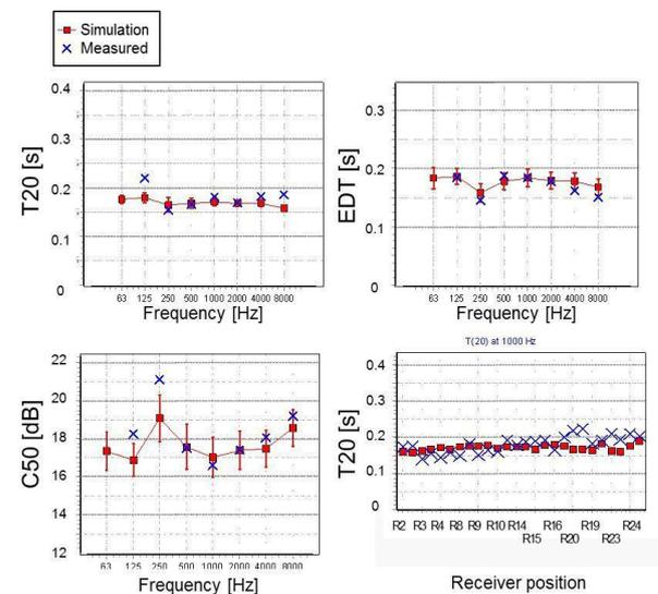
Figure 6. Comparison between measurements and simulation results
