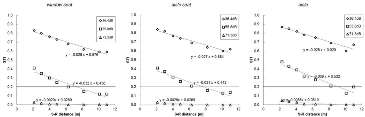
Figure 7. STI values of three receiver lines under three background conditions
