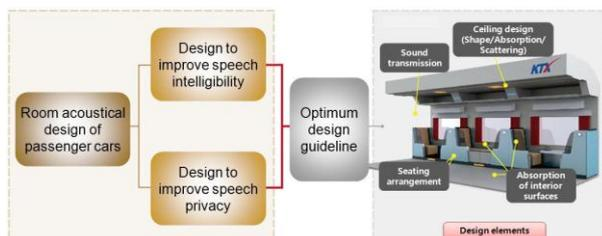
Figure 1. Research target and design elements in the high-speed train passenger cars
