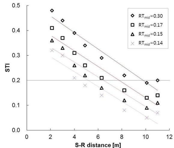
Figure 8. STI values with changes in absorption coefficients of interior surfaces
