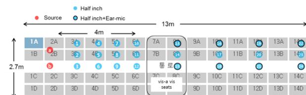
Figure 4. Microphone positions in the 2<sup>nd</sup> class passenger car of KTX
