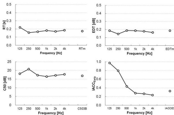
Figure 5. Acoustic measurement results in the 2<sup>nd</sup> class passenger car
