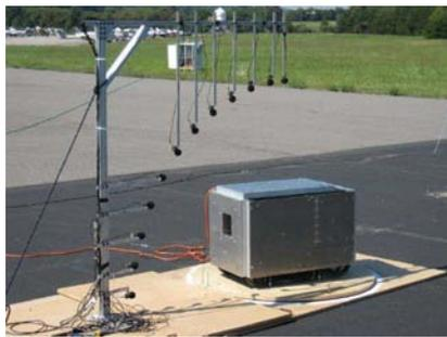
Figure 3. MTG with passive enclosure under noise testing.
