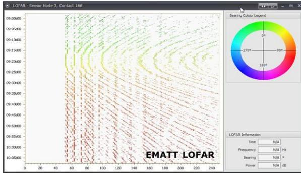
**Figure 8.** Example of processed sonar data of AUSSNet detected target at TS11, acoustically relayed.
