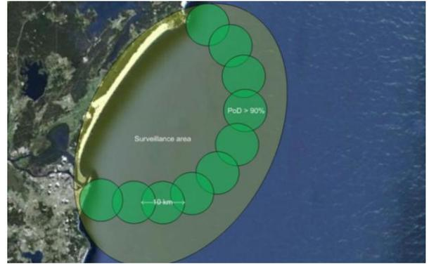
**Figure 10.** Sensor Network deployment for coastal surveillance in a ‘string’ network.
