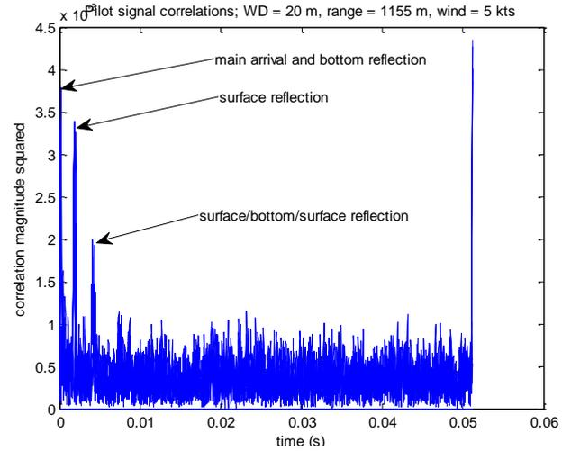
**Figure 5.** Multipath reverberations, shown as received signal correlator output modelled for a shallow water case, with windspeed set to 5 knots: Multipath is strong and coherent.
