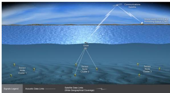
**Figure 9.** Cluster Network Access Node redundancy with multiple mobile gateways.
