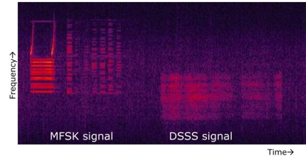
**Figure 3.** Channel probe followed by MFSK signal (left): received with many errors, and a DSSS signal with real-time channel probe (right): received with zero errors. Signals were recorded in 10 m water depth near Kiel, Germany. Range: 2-3 km
