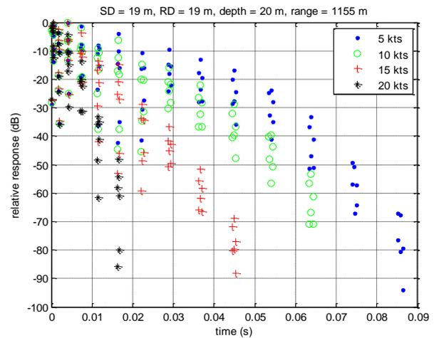
**Figure 6.** Modelled shallow water multipath level and delay spread variation with surface conditions (wind speed in kts)
