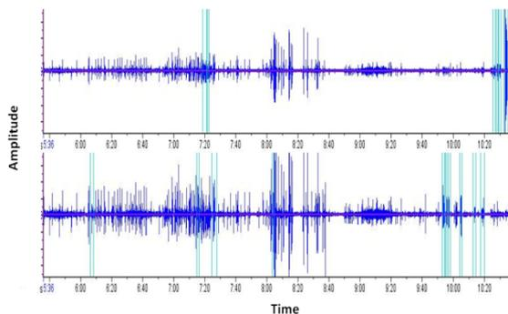
**Figure 5.** Time domain views of two hydrophone channels (#1 above, #2 below) of the 5 minute period prior to, and including, an exceptionally high amplitude 'thump' at the end of the 5 minute period. 'Thumps' are assigned to hydrophone channels based on received Sound Pressure Level.
