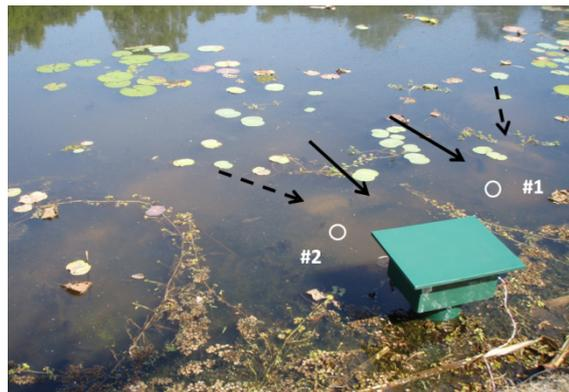
**Figure 1.** Playback study site water depth approx. 30 cm. Sound source is within green box and projects into the PVC tube pushed into the water and substrate. Tilapia are shown (solid arrows), nests (dashed arrows) and hydrophone positions (#1 and #2 as circles).
