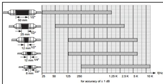
**Figure 4:** Typical intensity probe spacer selection (from Larson Davis Incorporated, 1999)
