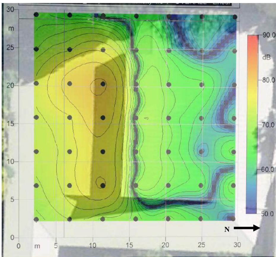
Figure 6: Rooftop sound power noise contour map
