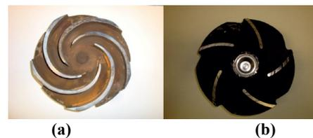
**Figure 3.** Impeller a) front, b) back (Wang, 2012)
