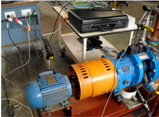
**Figure 4.** Photo of rig showing lasers focussing on motor shaft (left laser, B&K) and impeller shaft (right laser, Dantec). The rubber coupling is guarded by the orange shroud. The drive motor is at the left hand end and the volute at the right hand end of the image.
