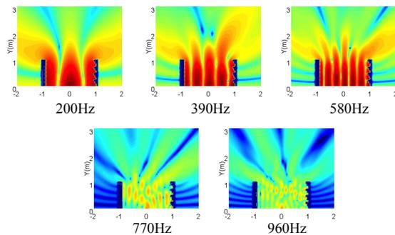
**Figure 4** Sound pressure distributions at the dips of the Insertion Loss curve of double barriers with a WTB at the right side.
