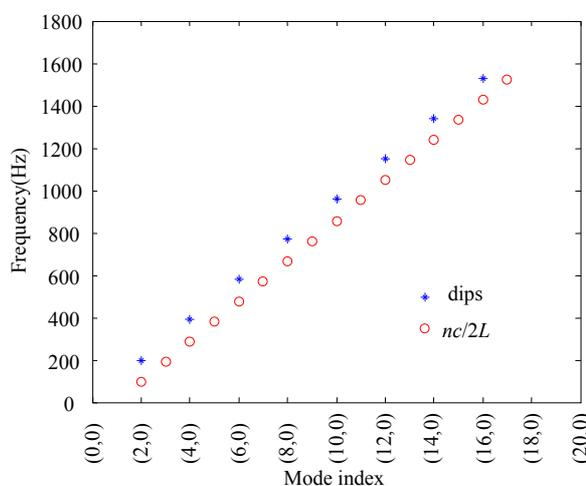
**Figure 3** Resonances of rigid cavity and the dip frequencies in the IL curve of double barriers.
