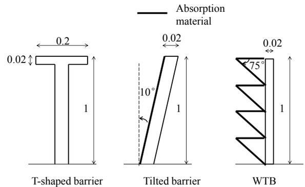
**Figure 5** Configurations of T-shaped, Tilted and WTB barriers.
