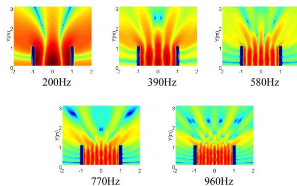
**Figure 2** Sound pressure distribution at first five dips of the Insertion Loss curve of double barriers.
