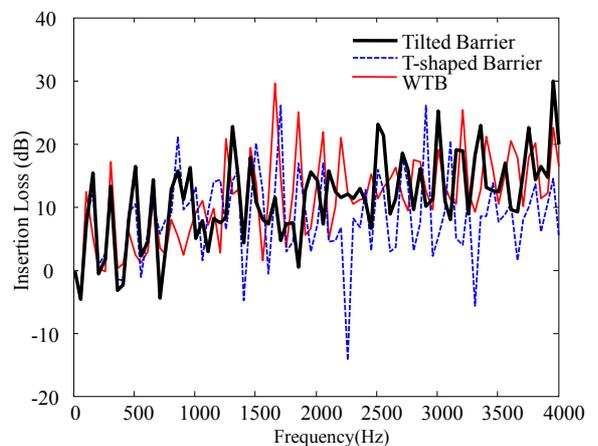
**Figure 6** Insertion Loss of three different types of barriers.
