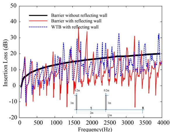
**Figure 1** Insertion Loss (IL) of single rectangular barrier, double rectangular barriers and WTB at right side barrier.
