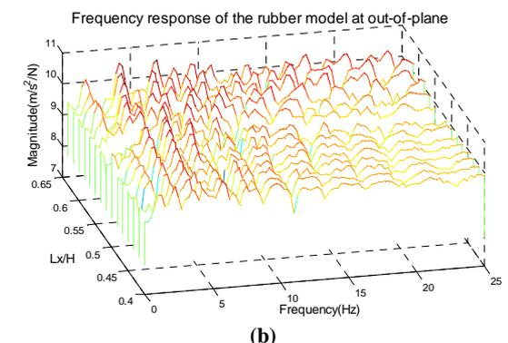
Figure 3: In-plane (a) and out-of-plane (b) frequency response functions of the model risers.
