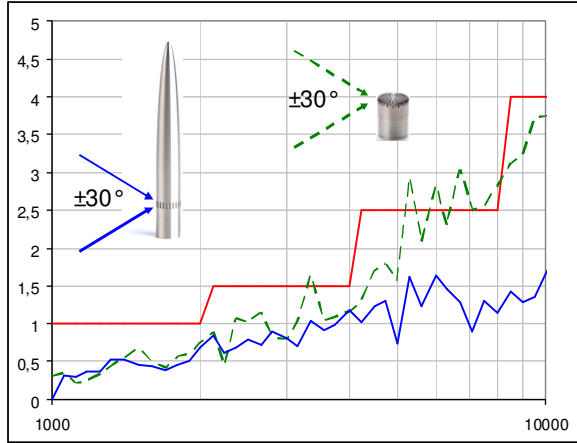
Figure 7. Directional response of DUO with acoustic cone (blue) for \theta = 30^\circ (reference direction 90^\circ ); Tolerance values of IEC 61672-1 (red) without expanded uncertainty.
