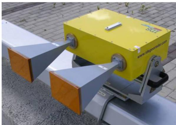
Figure 9. IBIS-S displacement measurement system
