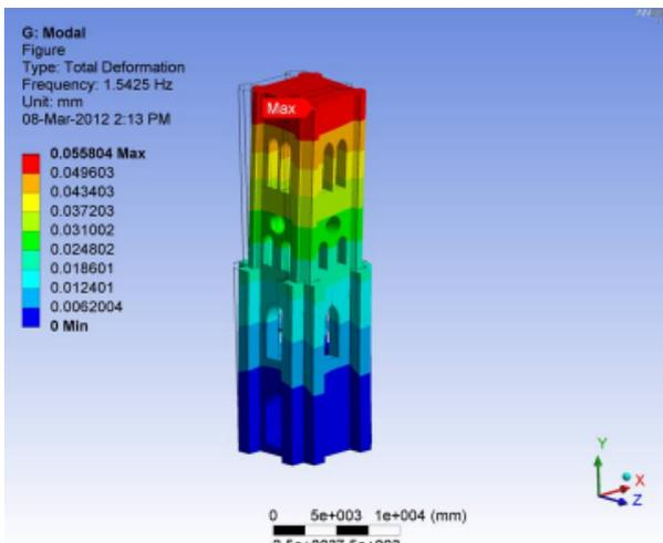
Figure 15. Fundamental bending mode (Y-Z direction)
