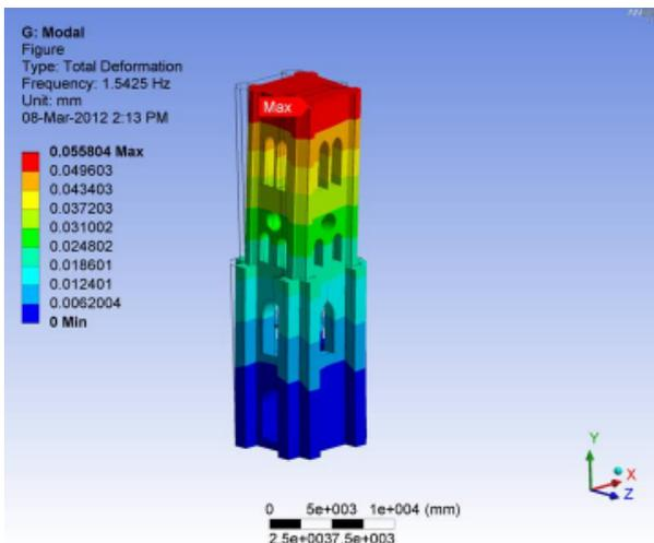
Figure 15. Fundamental bending mode (Y-Z direction)
