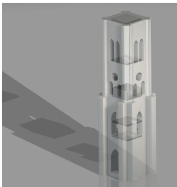
Figure 11. Geometry of the FE model
