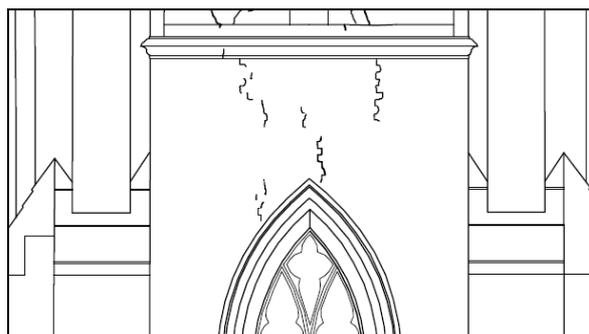
Figure 12. Sample plot showing documented cracks
