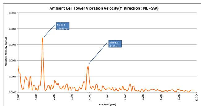
Figure 4. Sample ambient vibration spectrum (Y-Z Plane)
