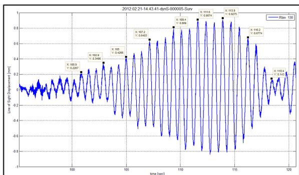
Figure 10. Sample IBIS-S displacement measurement
