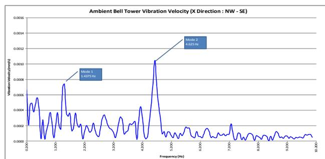
Figure 3. Sample ambient vibration spectrum (X-Z Plane)
