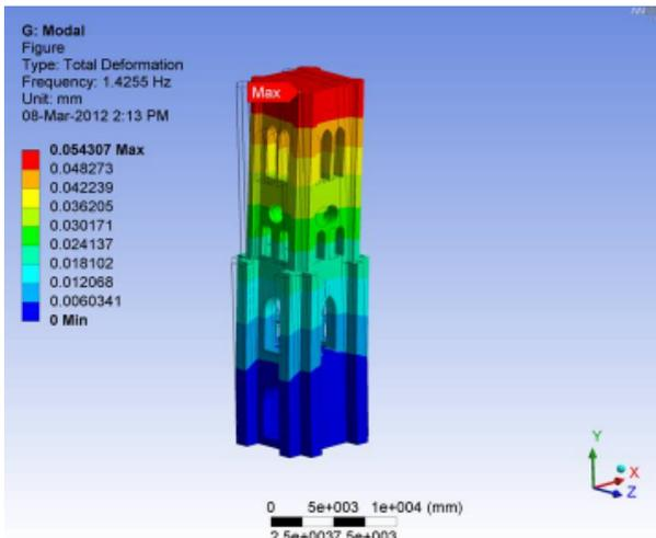
Figure 14. Fundamental bending mode (X-Z direction)
