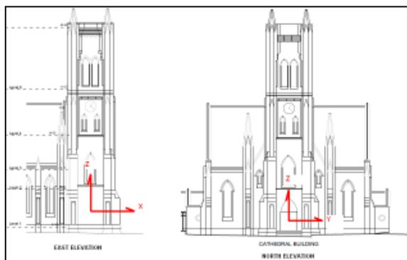
Figure 2. Elevations showing co-ordinate system
