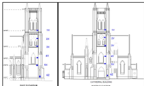
Figure 1. Accelerometer installation locations
