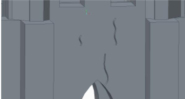
Figure 13. View of FE model showing simulated cracks
