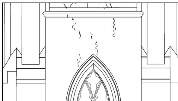
Figure 12. Sample plot showing documented cracks
