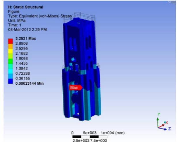
Figure 15. Stress contours from FE model dead load analysis
