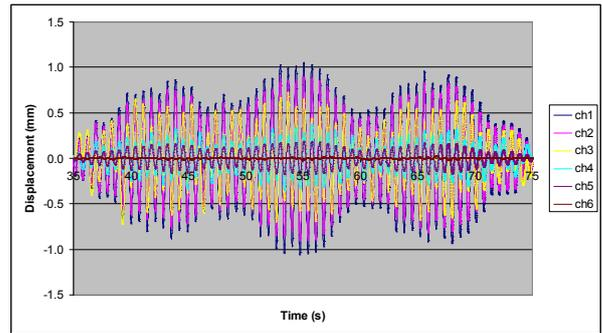
**Figure 8.** Mode 2 (1.5 Hz) – fundamental Y-Z sway mode
