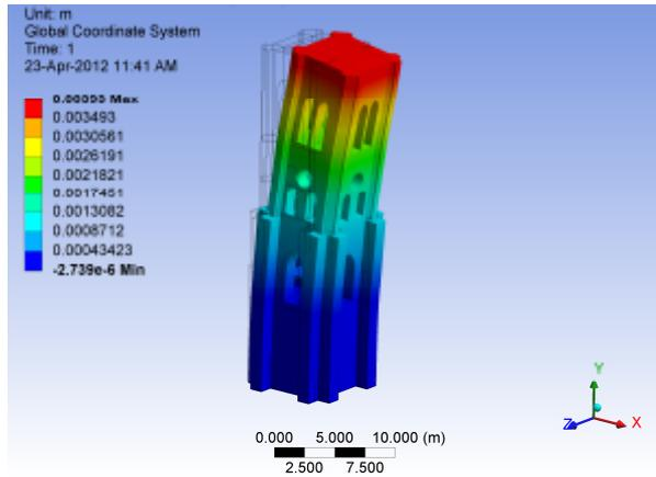
**Figure 5.** Mode 1 (1.4 Hz) – fundamental X-Z sway mode
