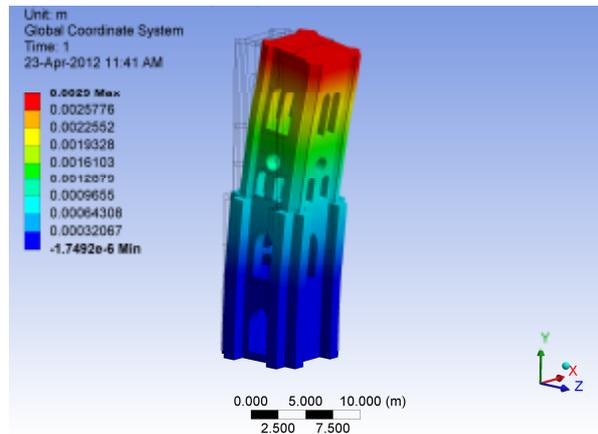
**Figure 6.** Mode 2 (1.5 Hz) – fundamental Y-Z sway mode
