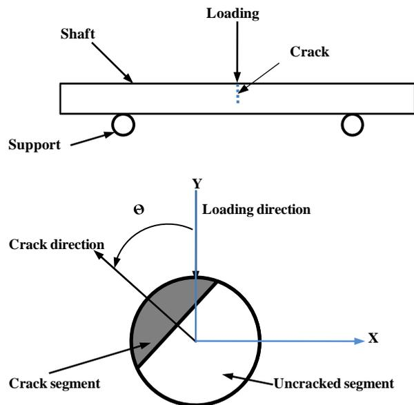
Figure 2. Top: a schematic diagram of the loading direction in three point bending test; bottom: Cross-section view at crack showing crack angular position.
