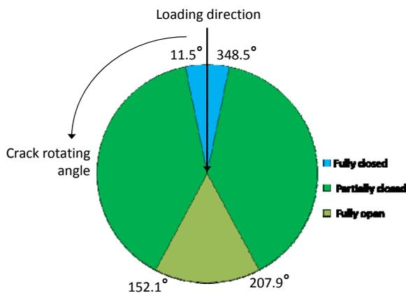
Figure 7. Relationship between crack angular position and its opening/closing status.
