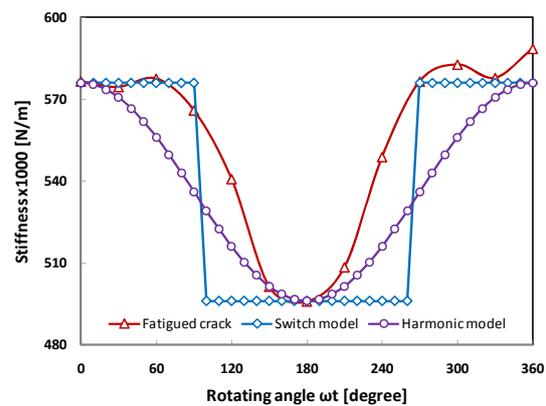
Figure 8. A comparison of measured periodic stiffness values and those calculated using theoretical models.
