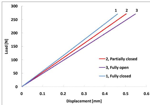
**Figure 3.** Loading force as a function of displacement for a fatigue-cracked shaft at three crack angular positions.
