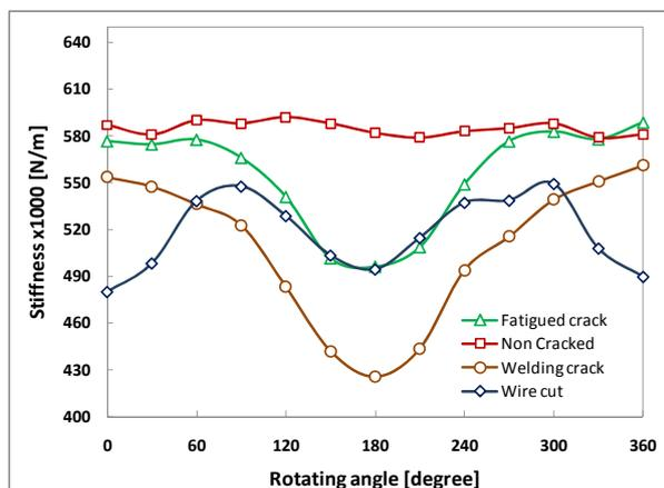
**Figure 4.** Bending stiffness at middle span for four shafts at various angular positions.
