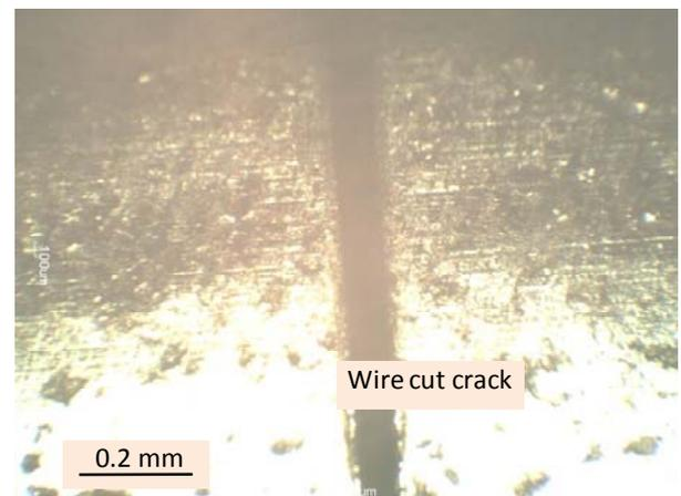
**Figure 6.** Wire cut crack observed under Moticam 2300 microscope.
