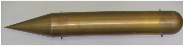
Figure 10. Air-filled brass cylinder
