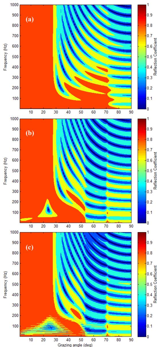
**Figure 2.** Plane wave reflection coefficient versus grazing angle and frequency from a layered shallow water seafloor system with geoacoustic parameters given in Table 1. Panel (a) considers the model without elastic properties in both sediment and substrate layers, Panel (b) without elastic properties in sediment layer, and Panel (c) with elastic properties in both sediment and substrate layers.
