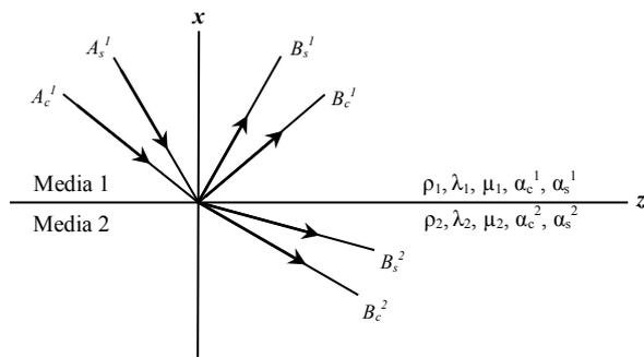
**Figure 1.** Elastic waves reflection and transmission at a boundary of two elastic half-spaces.
