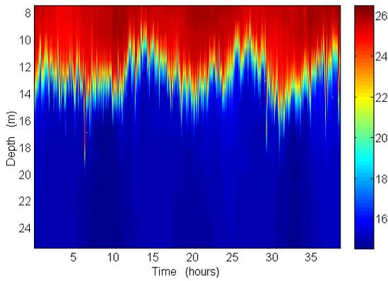
**Figure 2.** Temperature variation near the receiving hydrophones (40 hours)
