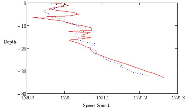
**Figure 9** SVP (m/sec) calculated for a single down and up-cast from a glider measuring temperature, salinity and depth (m). The solid red curve is the downcast and the dotted blue curve the upcast
