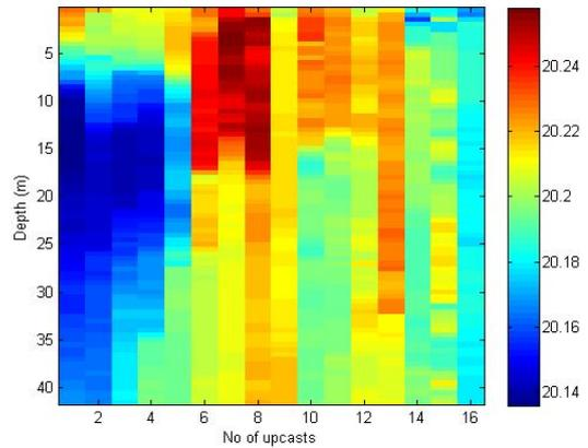
**Figure 12** Sequence of contiguous upcast temperature profiles (°C) as a function of depth
