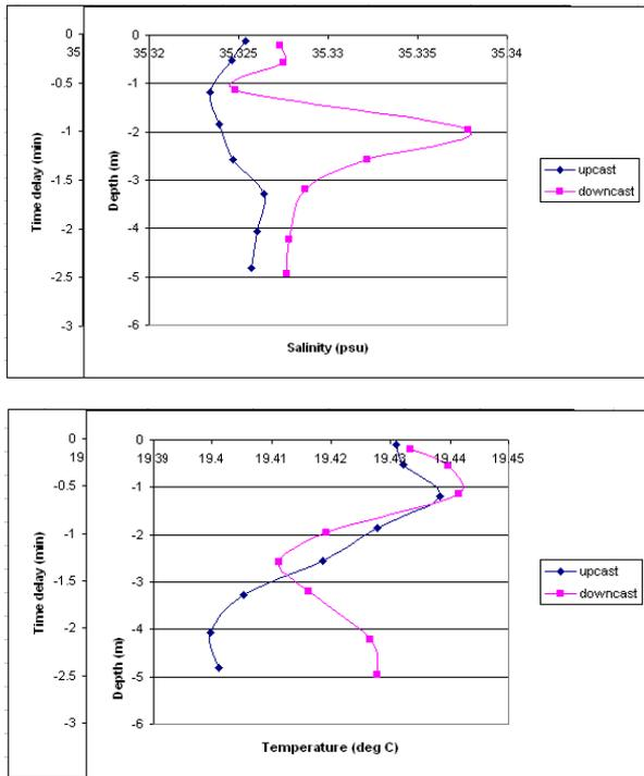
**Figure 11** Near surface salinity and temperature profiles as a function of depth and time delay between measurements at a given depth
