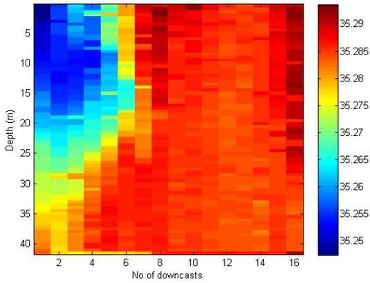
**Figure 15** Sequence of contiguous downcast salinity profiles (psu) as a function of depth
