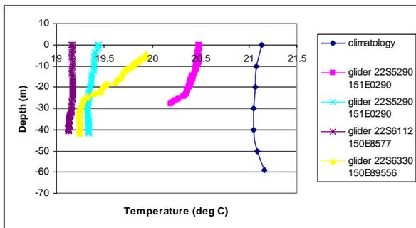
**Figure 8** Comparison between the temperature profiles recorded at different glider locations against climatology database
