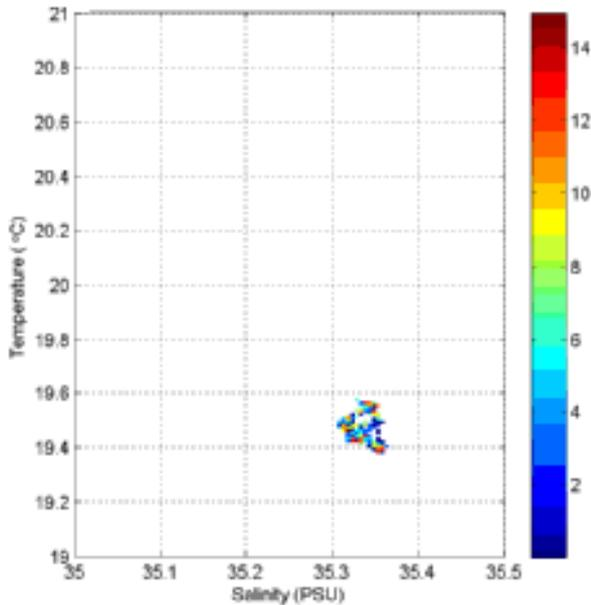
**Figure 4** TS diagram of well mixed water based on 1 hour of data. The colour intensity scale shows the number of points which recorded each temperature salinity pair
