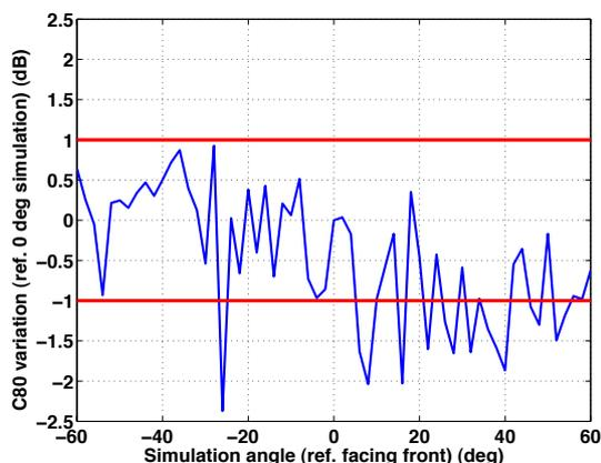
**Figure 7.**  $C_{80}$  variation for the simulated OBRIRs in blue expressed as the difference in dB from the 0 degree measurement. JNDs in two directions are shown in red.
