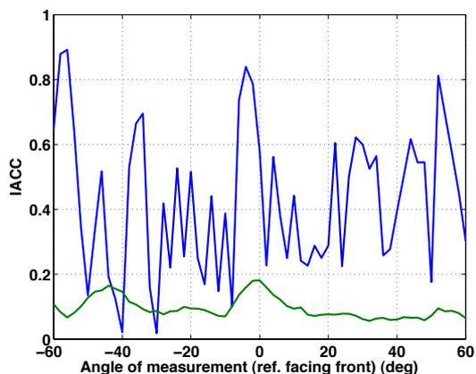
**Figure 9.** IACC of the measured room in green and simulated room in blue.
