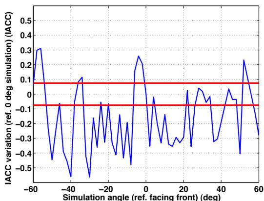
**Figure 8.** IACC variation for the simulated OBRIRs in blue express as the difference in IACC from the 0 degree measurement. JNDs in two directions are shown in red.
