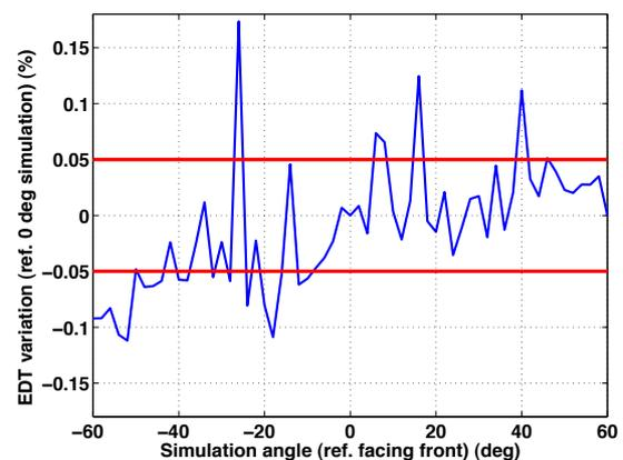
**Figure 6.** EDT variation for the simulated OBRIRs in blue as a percentage of deviation from the 0 degree measurement. JNDs in two directions are shown in red.
