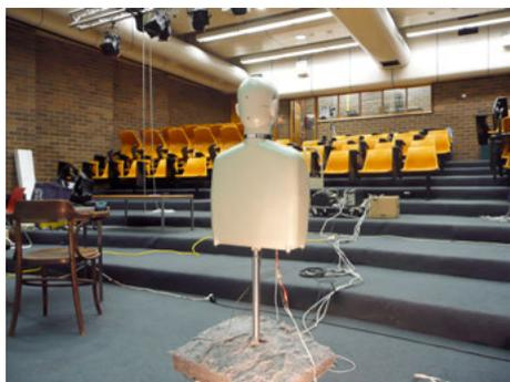
Figure 2. The location of the HATS in the real room used in the OBRIR measurement. The same location was used in the computer model in ODEON with the HATS mouth height of 1.5 m from the floor.
