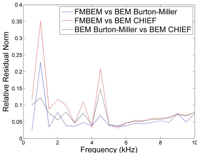
**Figure 3:** Plot of the relative residual norms versus Frequency between the FMBEM and commercial software results for the total surface pressure on the damping plate.
