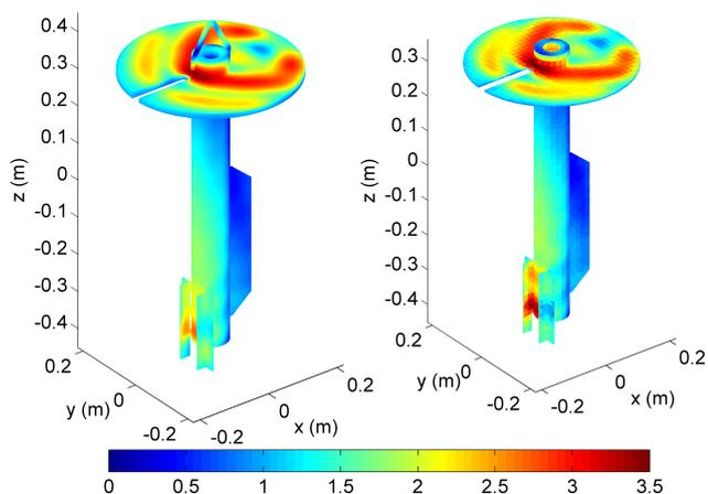
**Figure 2:** Comparison of high resolution (left) and low resolution (right) damping plate models. The colour variation indicates the total surface pressure in Pascals for a 10kHz unit strength incident plane wave.
