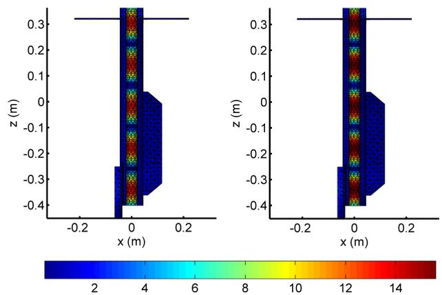
**Figure 5:** Comparison of the FMBEM (left) and CHIEF BEM (right) calculated total surface pressure for a 4.5kHz unit strength incident plane wave shown in the plane of symmetry for the low resolution damping plate model. The colour variation indicates the total surface pressure in Pascals.
