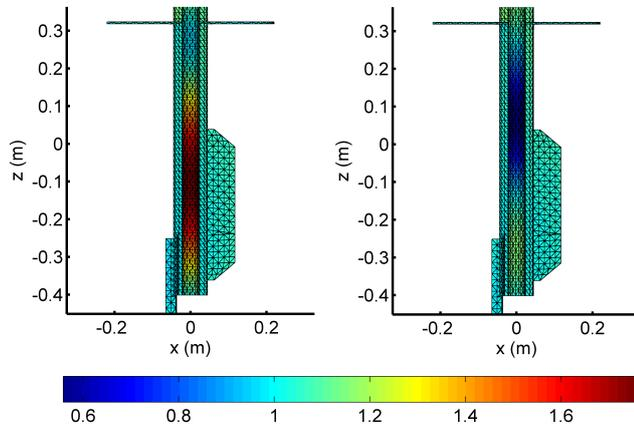
**Figure 4:** Comparison of the FMBEM (left) and CHIEF BEM (right) calculated total surface pressure for a 1kHz unit strength incident plane wave shown in the plane of symmetry for the low resolution damping plate model. The colour variation indicates the total surface pressure in Pascals.
