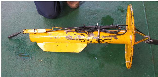
**Figure 1:** A photo of the hydrophone (black cylindrical shape) attached ready for deployment to the steel weight and damping structure (yellow).
