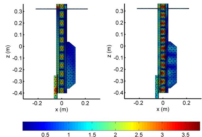
**Figure 7:** Comparison of the rigid (left) and coupled (right) FMBEM results for the calculated total surface pressure shown at 10kHz for a unit strength incident plane wave. The colour variation indicates the total surface pressure in Pascals.
