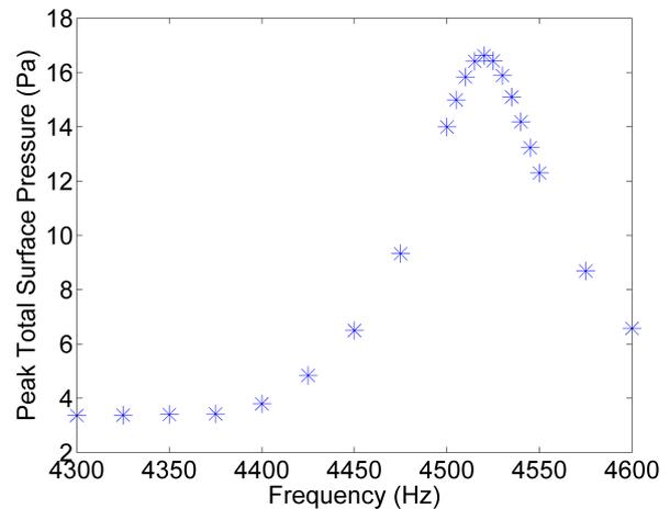
**Figure 6:** Plot of the peak total surface pressure versus frequency for the low resolution damping plate. The incident field again had an amplitude of 1 and was directed 45 degrees below the x-axis in the xz-plane.
