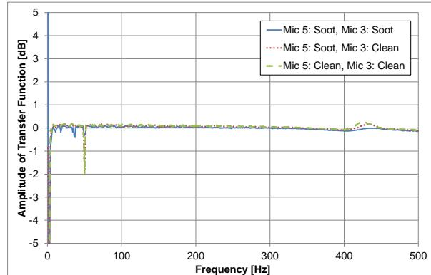
**Figure 15.** Amplitude of the transfer function between microphones with and without soot on the face.
