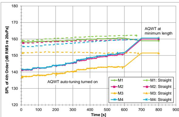
**Figure 13.** Measured SPLs over time at microphones M1 to M4 for a constant engine speed of 1800rpm. Beginning with 60kW applied load, a continual load of 7kW/min was applied over 10 minutes (resulting in 130kW). The EGT increased from 344°C to 452°C.
