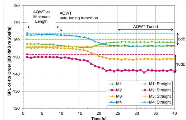
**Figure 10.** Comparison of with (solid line) and without (broken line) a AQWT installed in the exhaust system. When AQWT installed: variation from minimum length to tuned. Engine at 1500rpm, 106kW load, EGT 450°C
