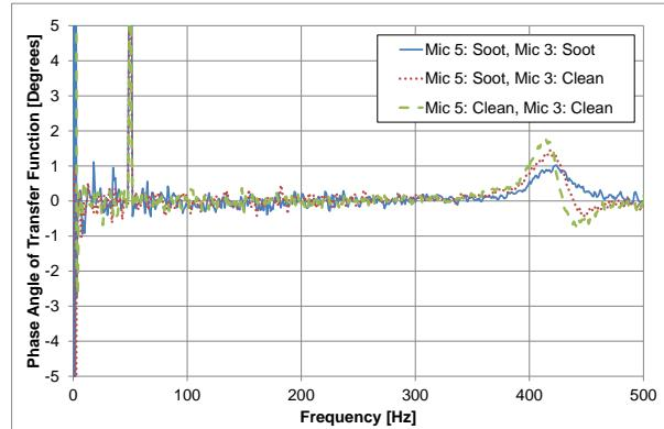
**Figure 16.** Phase angle of the transfer function between microphones with and without soot.
