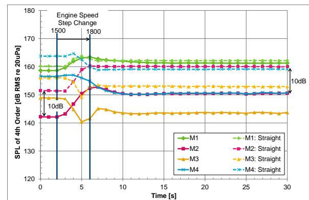
**Figure 11.** Measurement of SPL over time for a step change in engine speed from 1500rpm to 1800rpm, for both with an AQWT (solid line) and with a straight pipe (broken line). A constant EGT of approx. 450°C was maintained.
