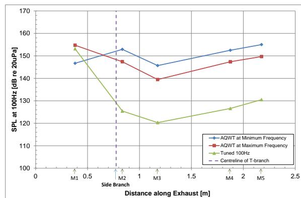
**Figure 8.** Sound Pressure Level at 100Hz for distances along the exhaust pipe for a constant engine speed of 1500rpm. No load was applied to the engine and the EGT at the side-branch was 163°C.
