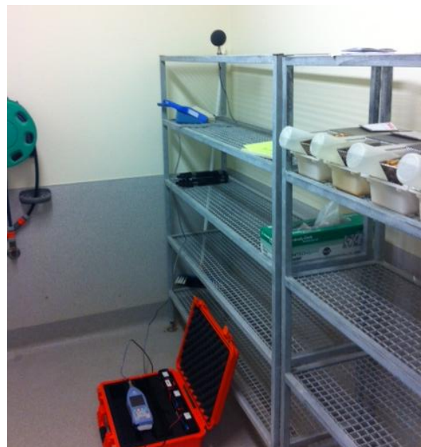
Figure 2: Rion NA-28 noise logger setup in Room 148
