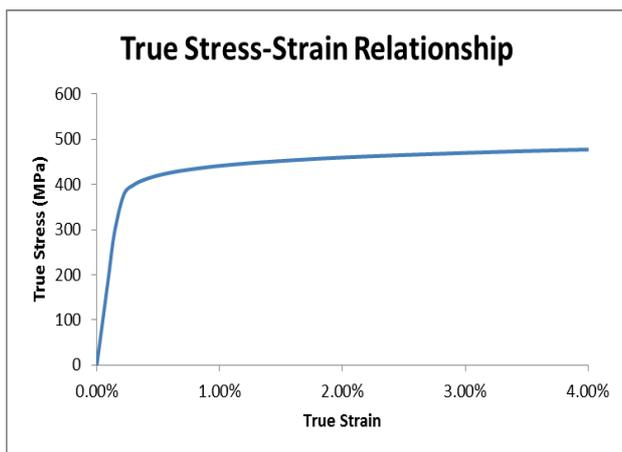
Figure 9. True Stress-Strain Curve
