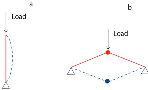
**Figure 2.** Buckling Schematics: (a) Symmetric Bifurcation
