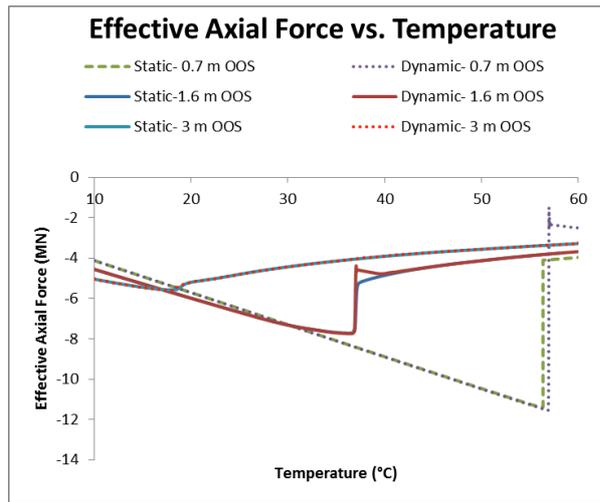
Figure 23. Effective Axial Force versus Temperature
