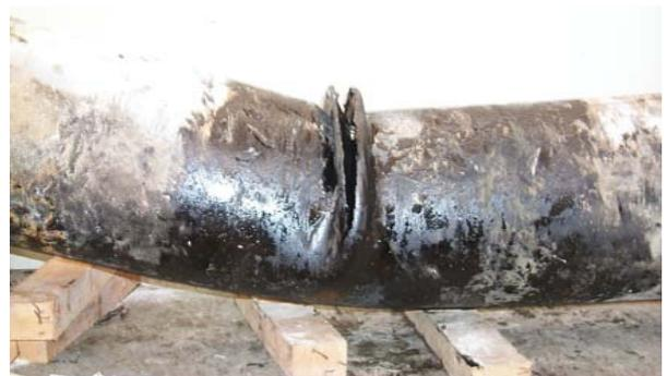
Figure 7. Example for Rupture Failure Mode under Bending (Palmer)
