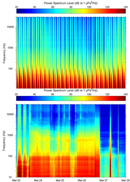
Figure 13. Spectrograms of recorded sound levels, Bay of Fundy, March 2012. Top: data from hydrophone internal to the HFM. Bottom: data from M8E hydrophone outside the streamlined float mooring. After 15 h the first mechanical failure of the float-frame occurred, followed by the complete plastic failure of the frame several days later.
