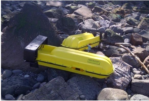
Figure 12. Failed streamline float.
