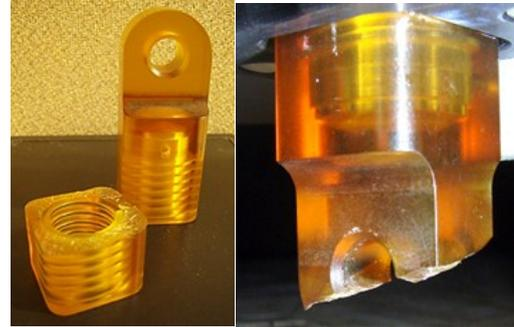
Figure 8. Left: Release block failure from shock loading during first deployment. Right: Fractured release block from second deployment.
