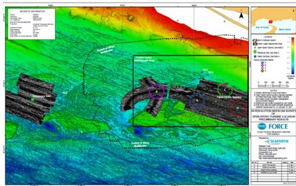
Figure 6. Bathymetry of FORCE Project and reference site.
