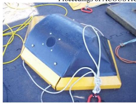
**Figure 3.** JASCO's high-flow mooring (HFM). The circular window in the cover is acoustically transparent.
