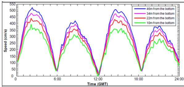
Figure 5. Current profile at Minas Passage, 7 May 2008 (Oceans Ltd. 2009).
