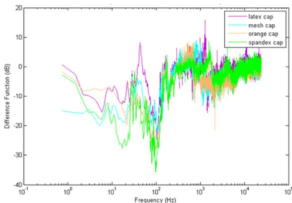
**Figure 2.** Measured sound spectra with various flow shield materials at 0.8 m/s flow.
