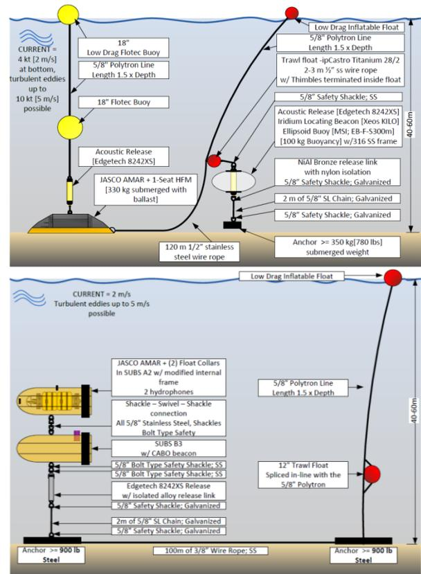
**Figure 11.** Modified high flow mooring (top) and stream-
