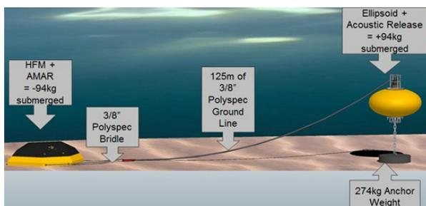
Figure 7. Mooring diagram for September and October 2011 deployments.
