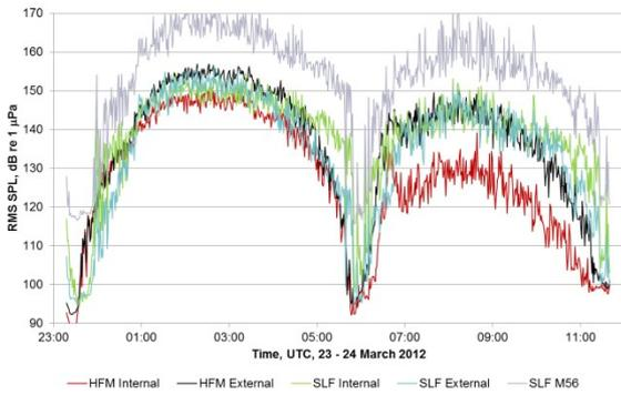
**Figure 15:** Comparison of RMS SPL levels all five hydrophones during the first full tidal cycle. The hydrophone internal to the HFM is significantly different from the other hydrophones during the ebb flow (06:00 – 12:00)
