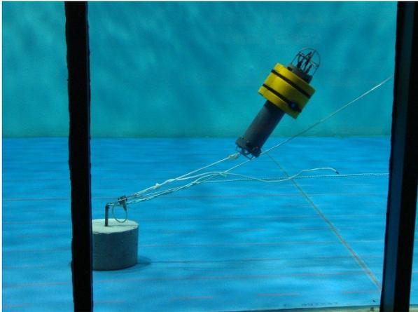
**Figure 1.** JASCO's Autonomous Multichannel Acoustic Recorder (AMAR) in a 0.8 m/s current in the flume tank at the Centre for Sustainable Aquatic Resources (CSAR) at Memorial University, St. John's, NL.
