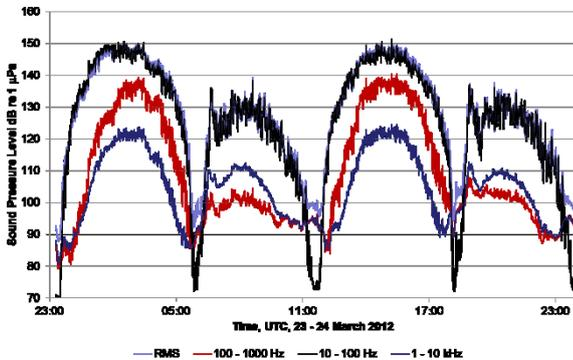
**Figure 16.** RMS and decade sound pressure levels for the hydrophone inside the flow shield of the high flow mooring for the first two tidal cycles. The noise in the band of 100 – 1000 Hz is 25 - 35 dB lower during the ebb flow than the flood.
