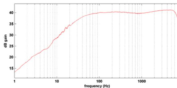
**Figure 2:** System gain curve of the first noise logger deployment.
