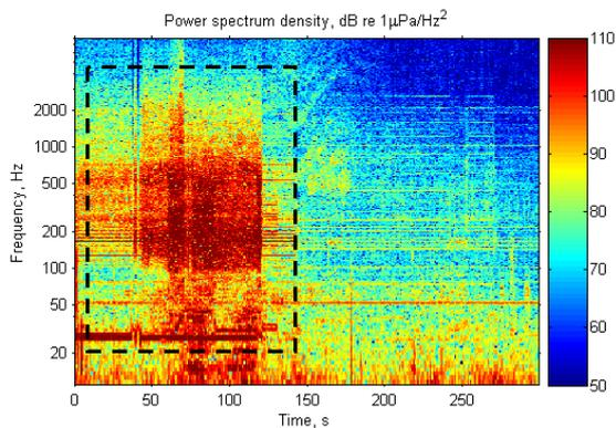
**Figure 5.** Spectrogram of underwater noise from a train passing over a nearby bridge (demarcated by the dashed lines).
