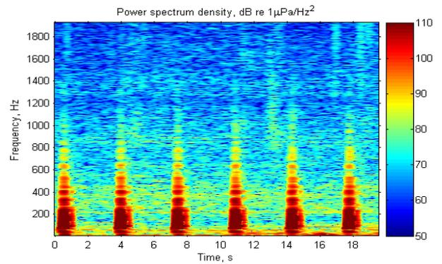
**Figure 7.** Spectrogram of noise from impact pile driving.
