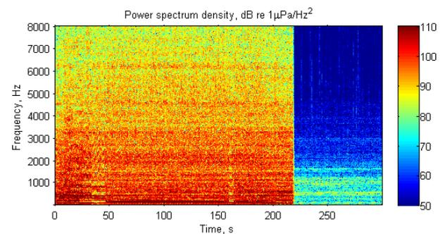
**Figure 8.** Spectrogram of noise from vibratory pile driving.
