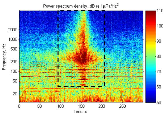
**Figure 6.** Spectrogram of noise from a vessel passing (demarcated by the dashed lines).
