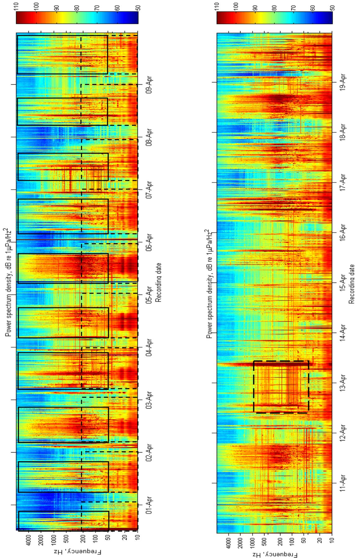
**Figure 3.** Spectrograms of noise sources during the period from the 31<sup>st</sup> of March to the 19<sup>th</sup> of April, 2010. In the top figure, examples of periods of frequent train noise (dashed lines) and periods of frequent vessel noise (solid lines) are demarcated. In the bottom figure, an example of continuous machinery noise is demarcated (dashed lines).
