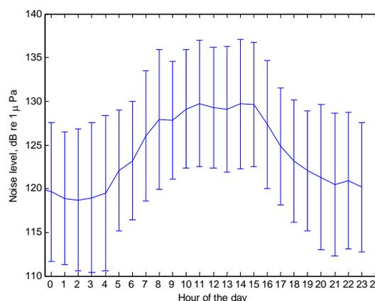
**Figure 12.** Mean broadband (10-4500 Hz) noise level versus hour of the day, error bars show one standard deviation.
