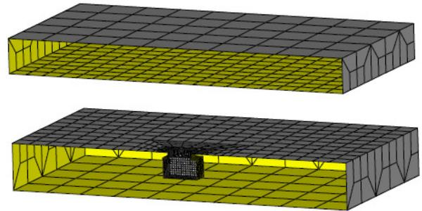
Figure 3. Open resonator consisting of two parallel plates with a Helmholtz resonator embedded in the lower plate
