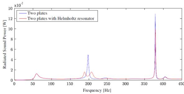
**Figure 4.** Radiated sound power by the open resonator consisting of two parallel plates with an oscillating upper plate – with and without a Helmholtz resonator embedded in the lower plate
