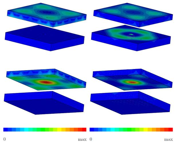
**Figure 6.** Normalized normal sound intensity (left) and surface contribution (right) for the two parallel plates with a Helmholtz resonator at 198 Hz
