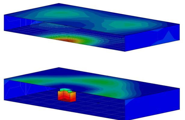
**Figure 7.** Section view of the two parallel plates with a Helmholtz resonator showing the normalized continuous surface contribution at 198 Hz
