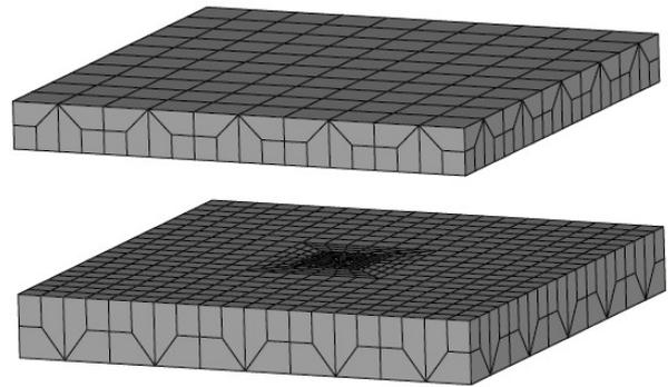
Figure 2. Open resonator consisting of two parallel plates
