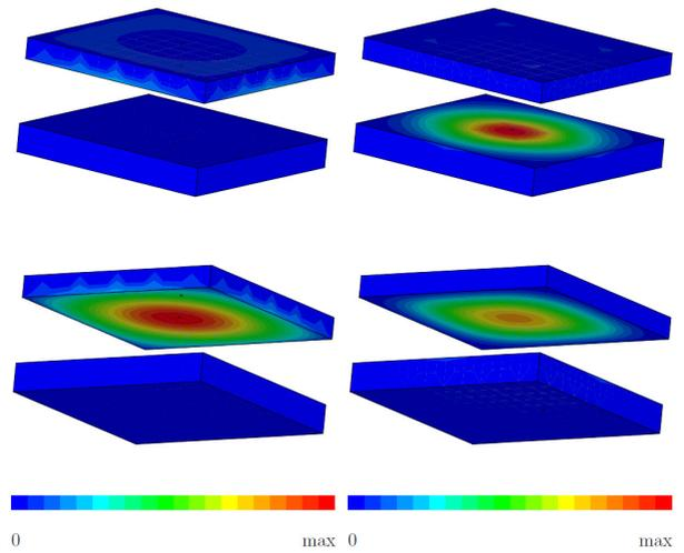
**Figure 5.** Normalized normal sound intensity (left) and surface contribution (right) for the two parallel plates at 198 Hz
