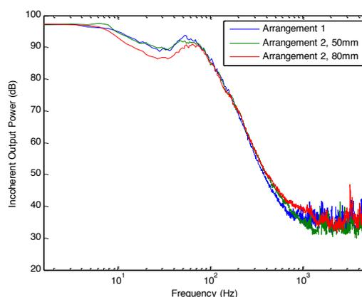
**Figure 15.** IOP comparison between two different microphone arrangements with a 45 mm windshield for airflow velocity of 16 m/s
