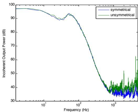
**Figure 10.** IOP between microphones for Arrangement 1 equipped with 45 mm windshield with airflow velocity of 16 m/s for symmetrical and asymmetrical positioning of microphones
