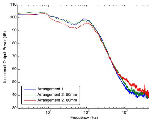
**Figure 16.** IOP comparison between two different microphone arrangements with a 45 mm windshield for airflow velocity of 28 m/s
