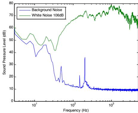
**Figure 2.** Sound pressure level of the response microphone for background and 106 dB white noise without the jet present and with microphones covered with a 90 mm windshield
