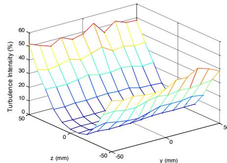
**Figure 5.** Turbulence intensity profile 200 mm downstream from the jet exit plane for free stream velocity of 6 m/s. Graph origin corresponds to the jet centreline.
