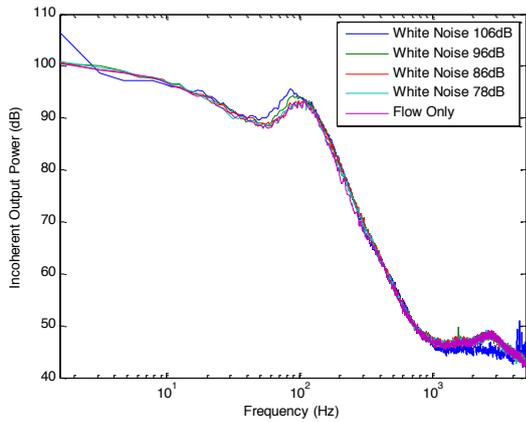
**Figure 9.** IOP between microphones positioned in Arrangement 1 and equipped with 60 mm windshields at airflow velocity of 28 m/s and different loudspeaker levels
