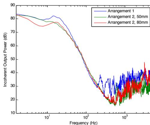
**Figure 14.** IOP comparison between two different microphone arrangements with a 45 mm windshield for airflow velocity of 4 m/s
