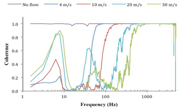
**Figure 6.** Coherence between microphones positioned in Arrangement 1 equipped with 90 mm windshield at selected airflow velocities of 4, 10, 20 and 30 m/s as well as with no flow
