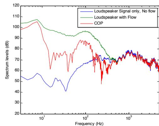
**Figure 19.** Auto spectra of a microphone in Arrangement 2 located in the jet with loudspeaker signal, with and without flow, as well as the COP between microphones in Arrangement 2 for a 45 mm windshield and airflow velocity of 28 m/s
