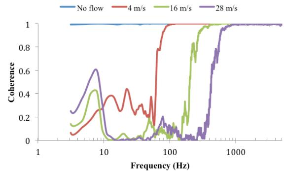
**Figure 7.** Coherence between microphones positioned in Arrangement 2 equipped with 45 mm windshield at selected airflow velocities of 4, 16 and 28 m/s as well as with no flow
