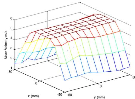
**Figure 4.** Mean airflow velocity profile 200 mm downstream from the jet exit plane for free stream velocity of 6 m/s. Graph origin corresponds to the jet centreline.
