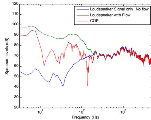
**Figure 18.** Auto spectra of a microphone in Arrangement 2 located in the jet with loudspeaker signal, with and without flow, as well as the COP spectrum between microphones in Arrangement 2 for a 45 mm windshield and airflow velocity of 16 m/s
