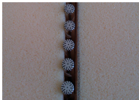
Figure 11 – Photo of array microphones with 60 mm thick Dunlop Enduro Foam (EN 38-200) wedged around microphones.
