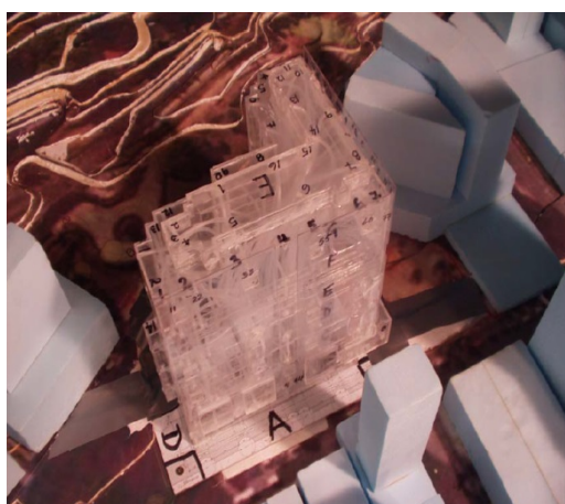
Figure 10 Wind tunnel model of the building with removable secondary façade
