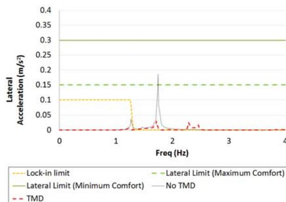
Figure 21 Reduction of lateral accelerations using vertical TMDs
