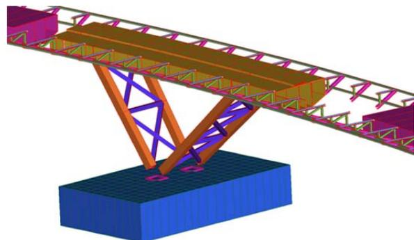
Figure 3 Detailed View of the V-Columns, OutRiggers and Box-Girder
