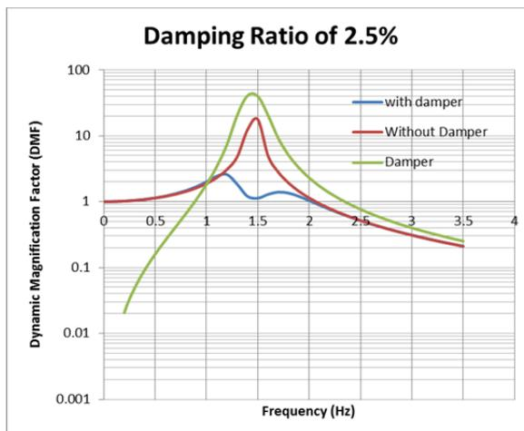
**Figure 18** DMF for structure with/without TMD and for the TMD itself
