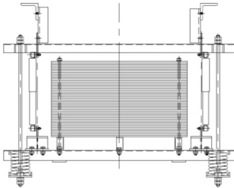
Figure 19 Tuned Mass Damper Design Drawing
