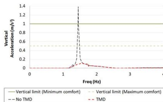
Figure 20 Reduction of vertical accelerations using vertical TMDs
