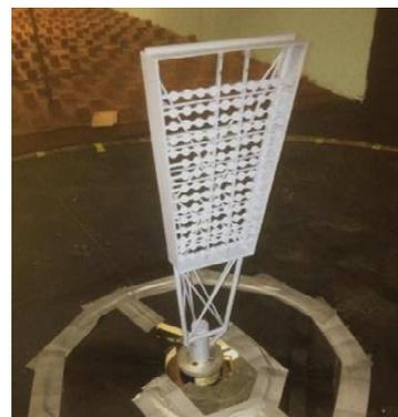
**Figure 11** Wind tunnel model of light tower headframe
