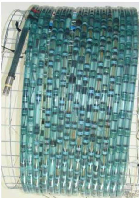
Figure 2. FOTA Array section wound on calibration drum
