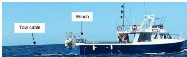
Figure 4. Support vessel towing the FO Array
