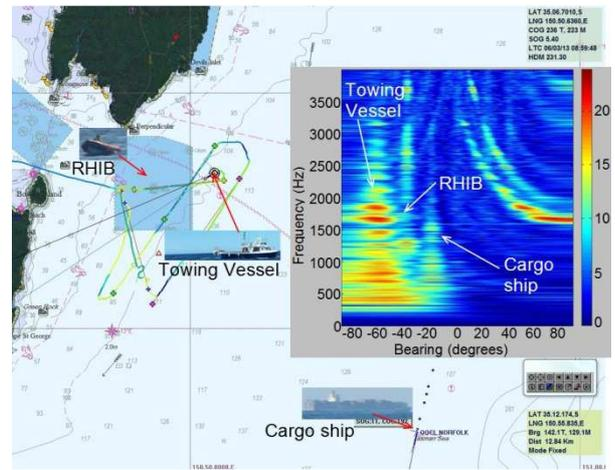
Figure 12. Detection of a commercial cargo ship and RHIB
